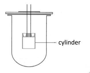
The "paddle mixer" device, in which the rotating mixer and shaft are replaced by a rotating cylinder made of stainless steel.
