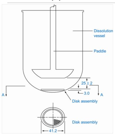
The paddle mixer, additionally equipped with a stainless steel prefabricated disc in the form of a mesh with a hole size of 125 microns.
