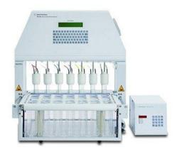
It consists of a set of cylindrical flat-bottomed glass vessels, a set of glass piston cylinders. The cylinders make vertical reciprocating movements inside the vessels filled with the dissolution medium, the speed of the cylinders (the number of drops per minute) is indicated in the normative document.
